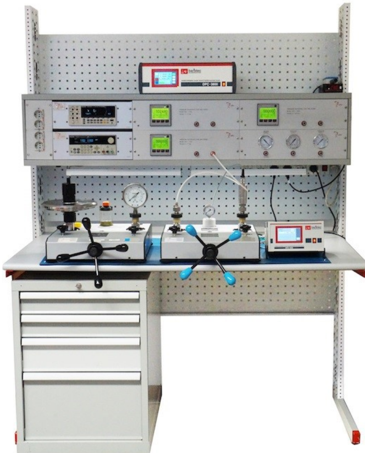
Pressure laboratory test bench
